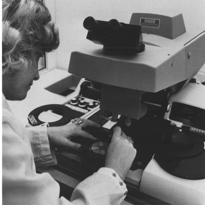
Cobalt Mask Aligner positions the patterns for placement of circuits on thin film heads. ➤
