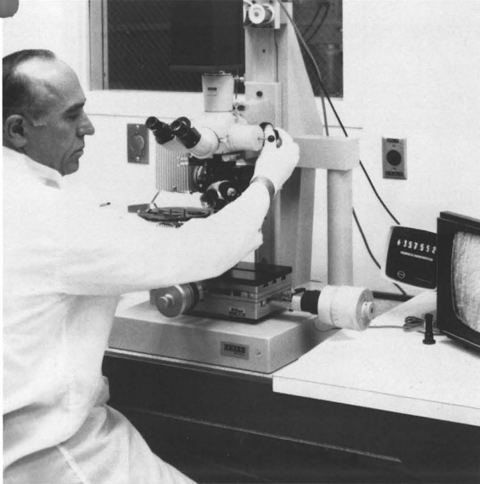
Advanced test equipment scans and analyzes rigid disc surfaces to micro-inch level. ➤
